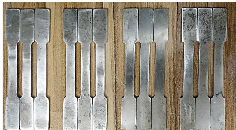
Figure 9. Tensile Test Specimens each three for specific group.
