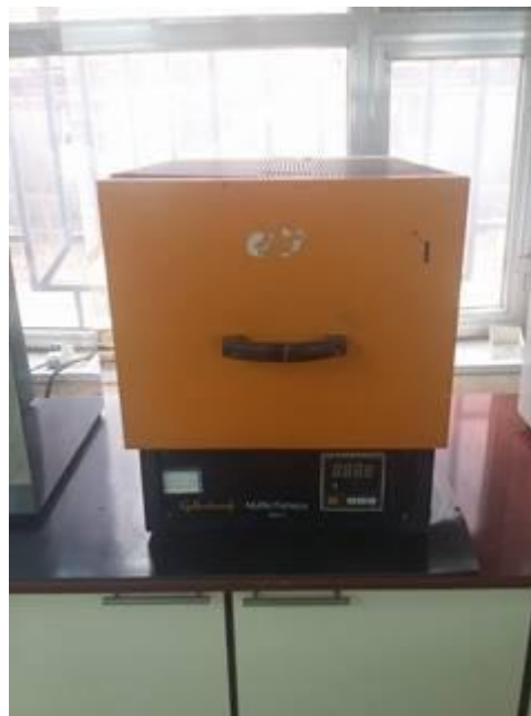
Figure 1. Show the electrical furnaces for heat treatment.
