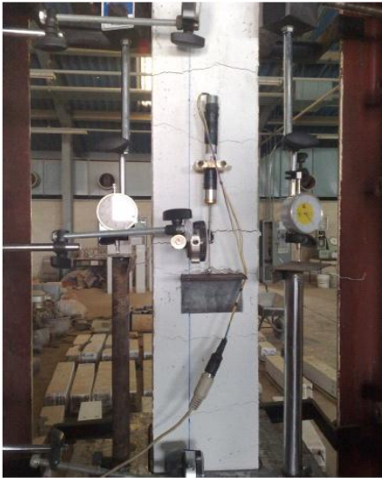
Figure 8. LVDT use to measure axial displacement.
